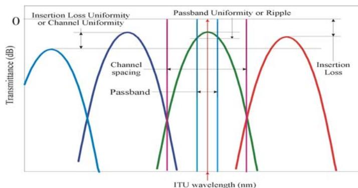
Fig. 8. Graphical representation of insertion loss, insertion loss uniformity, and passband uniformity.
