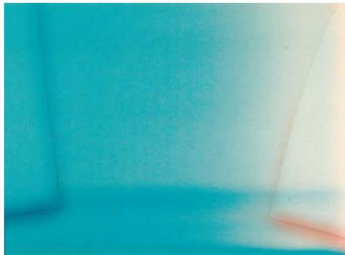
Fig. 7. Photomicrograph of the interface between the slab and array waveguides of an AWG chip (arbitrary magnification).
