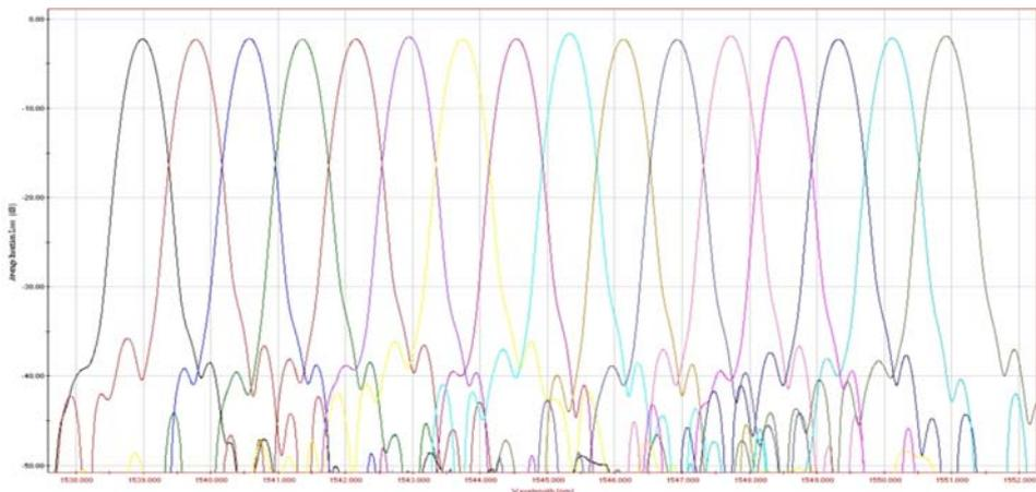
Fig. 8. Spectral response of a 40 channel arrayed waveguide grating (mid 16 channels shown here).
