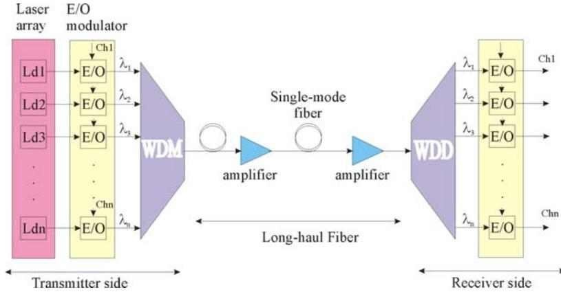
Figure 2. Basic structure of a point-to-point optical transmission system.
