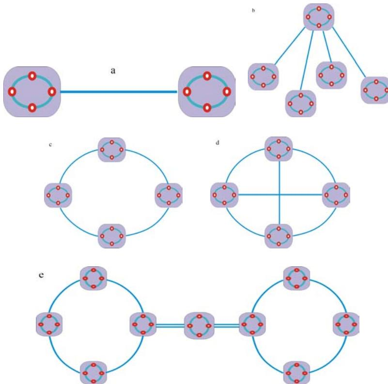
Fig. 3. Different WDM topologies. a) Point-to-point, b) Star, c) Ring, d) Mesh, e) Cross-connect.
