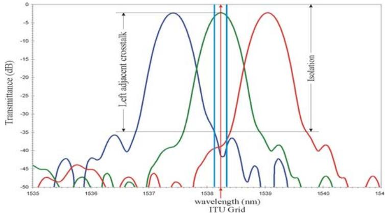
Fig. 9. Graphical representation of channel isolation and adjacent crosstalk.
