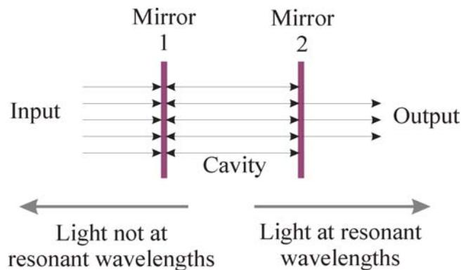
Fig. 4. Basic structure of a Fabry-Perot Etalon filter.
