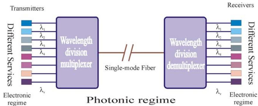
Fig. 1. Basic concept of WDM and WDDM in fiberoptic communications.
