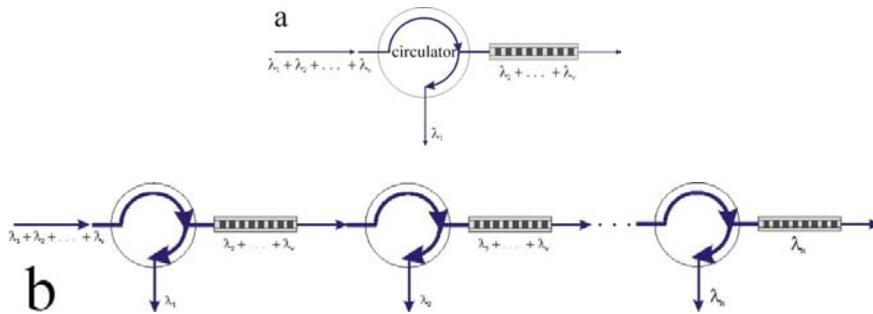
Fig. 6. a) Filtering a single wavelength from a multiplexed signal with an in-fiber Bragg grating. b) Basic structure of a DMUX by cascaded FBGs and circulators.
